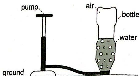
The air–water mixture is called the propellant.
